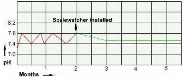
A graphic illustration of the actual reduction in Chlorine, whilst the graph shows the stability of pH, without the addition of chemicals, following the installation of the Scalewatcher at a municipal pool.
