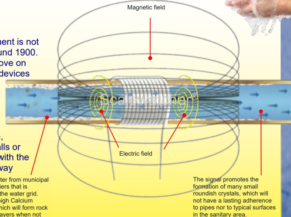
The signal promotes the formation of many small roundish crystals, which will not have a lasting adherence to pipes nor to typical surfaces in the sanitary area.
